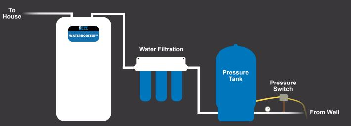
All existing components of the previous well system remain intact, including the pressure switch, pressure tank, and water filtration system. The Water Booster system will be seamlessly integrated into the plumbing system, positioned after the filtration system and prior to the building or house.
