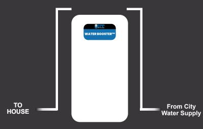
3. Take the line from the city water and the water line to the house. Plumb both of these water lines to the top of the Water Booster. 4. There are two open pipes on top of the system. One pipe is labeled with a sticker indicating "To House". Hook up the line that goes to the house to the outlet with the sticker labeled "To House". Hook up the line that comes from the city water source to the non labeled inlet.
